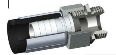
The connector with sealing cone is press-fitted into the end of the hose.
